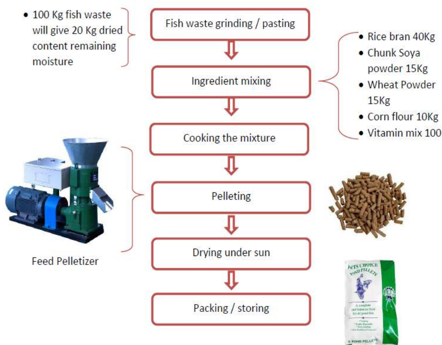
Figure 4. 8: Flow chart of fish pellet feed production by ICAR-CIFT
